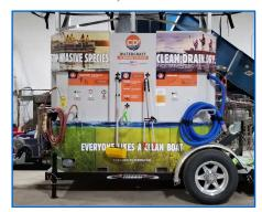
The theory behind the CD3 Boat Cleaning Station is to clean, drain, and dry boats. This makes the boats uninhabitable for AIS, as they need water to survive.
